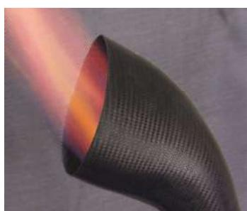
**PyroSic is a composite material specifically developed for lightweight structural parts exposed to heat or fire.** PyroSic composites are based on advanced glass-ceramic matrices (patented) reinforced with silicon carbide fibers. They feature a long-term temperature resistance of up to 650°C (1200°F). They can also be used at temperatures in excess of 1000°C (1800°F) on a short-term or intermittent basis.
